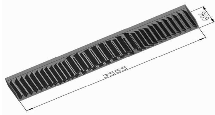
Fig. 3.14: View of the multigap RPCs distribution in the module box.
