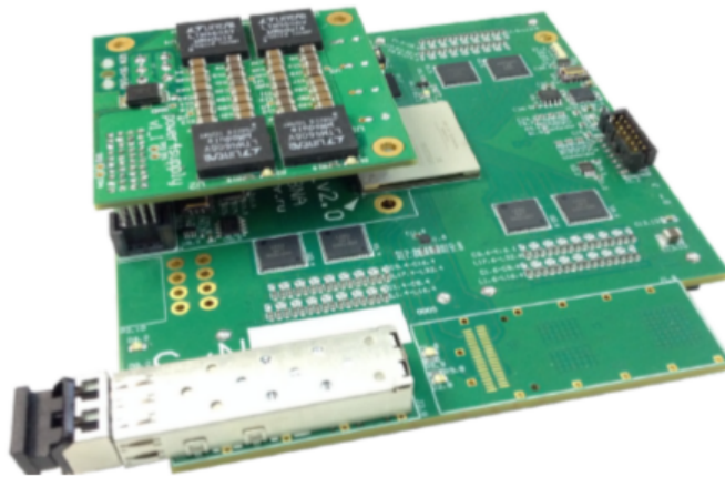
Fig. 54: The photo of ADC64s2 board planned for the FHCAL readout.
