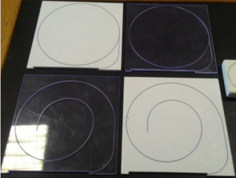
Fig. 41: Photo of scintillator tiles with different reflectors and different shapes of the grooves. Top left - tile with circular groove and chemical treatment of the scintillator surface, top right - tile with circular groove without reflector, down left - tile with spiral groove without reflector, down right - tile with spiral groove and chemical treatment of the scintillator surface.
