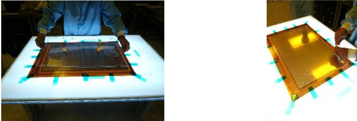
Figure 11.2: Assembly of detector based on 3 pc GEM-foils
