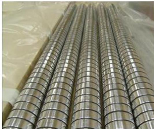
Figure 3.8: Potential degrader rods produced by industry using composite material (Kevlar + Macrolon + Al foil)
